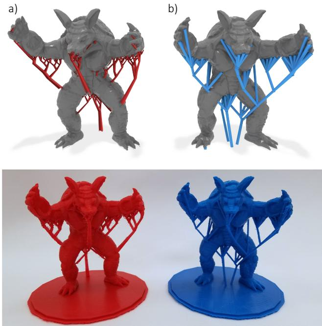
Fig. 12. **Armadillo supports.** PICO can automatically generate organic supports for 3D printing. We compared our generated supports (b) to the work of [68] (a). We used the same overhang points and same dimensions of the print and we achieved a comparable resulting weight of the used material.
