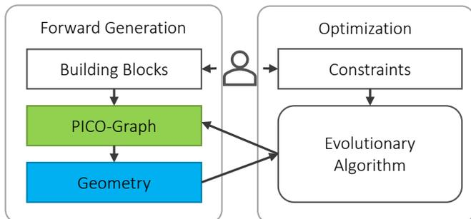
Fig. 2. Overview of PICO. User defines the *building blocks* which represent parameterized geometry generating operations with connectivity information. During the *Forward Generation* the user can connect the operations into a *PICO-Graph* that generates the output *geometry*. Alternatively, the user can define a set of *constraints* that are *optimized* for by an evolutionary algorithm. The constraints can be modified interactively while various geometries are generated and shown to the user.
