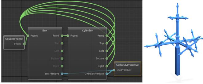
Fig. 5. An example of a PICO-Graph with cycles (left) and the generated recursive structure (right). Blue edges represent Constructive Solid Geometry (CSG) primitives and green edges 3D coordinate frames. The sink operation blends the incoming primitives and outputs them to the scene.
