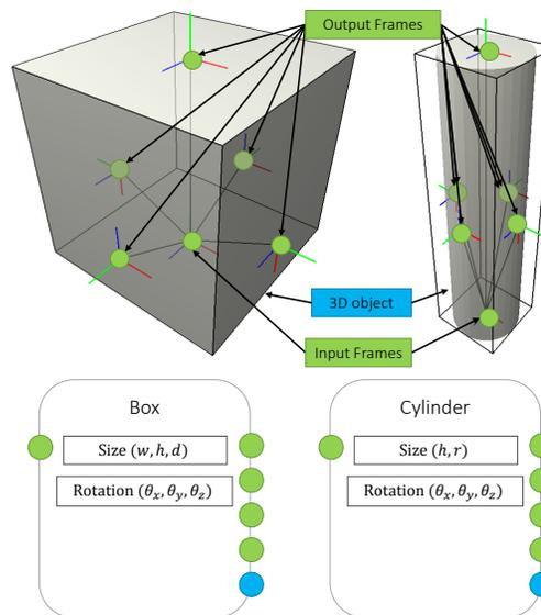
Fig. 3. An example of two building blocks generating a box and a cylinder respectively. The input and output frames can be positioned and orientated arbitrarily and define how the primitive will connect to others. The size and orientation with respect to an incoming frame are parameterized.
