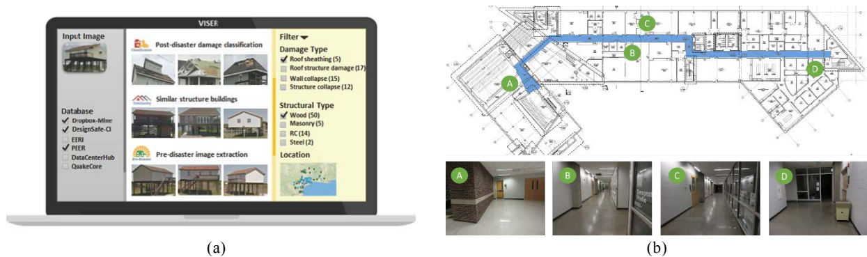
Fig. 7 – Future applications to produce VISER: (a) overall concept for Netflix-like search capability, an image is used to initiate the search, various databases are subscribed to, and similar images are provided; (b) automated reconstruction of path mapping for indoor reconnaissance missions, localizing images and linking them to locations on a structural drawing
