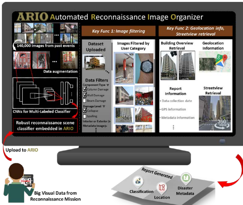
Fig. 1 – Overview of ARIO: Rapid, automated reconnaissance image classification, data sets uploaded from the field or the office over the web; report generation; and sorting and filtering.
